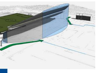
The seating bowl plan influences the elevation and section of the Stand. The curved bowl profile is visually apparant externally and is reflected in the shape of the 'back of tier' seating profile.
